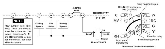
Figure 7. Typical Wiring Diagram for Heat/Cool, 4-Wire, Single Transformer Systems
